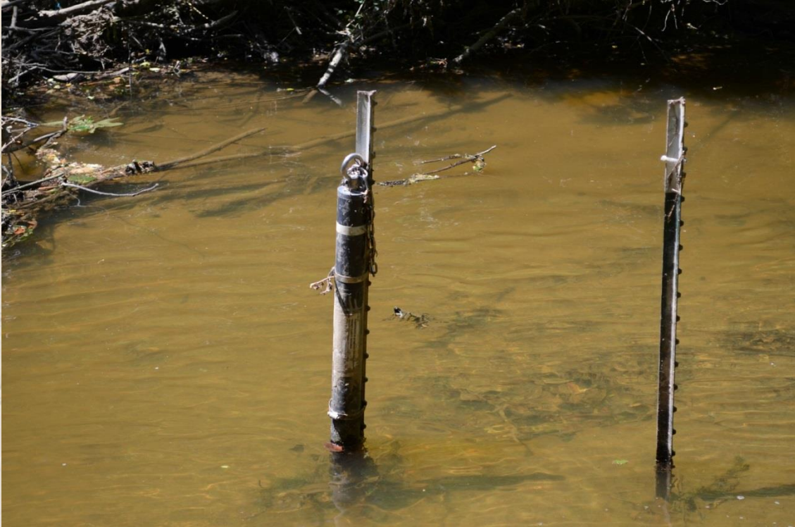
Figure 7: Part of AWRI's Project Clarity monitoring involves documenting the actual clarity of the water in the Macatawa River, which is the main source of water to Lake Macatawa. Turbidity sensors placed in the stream continuously measure turbidity levels.
