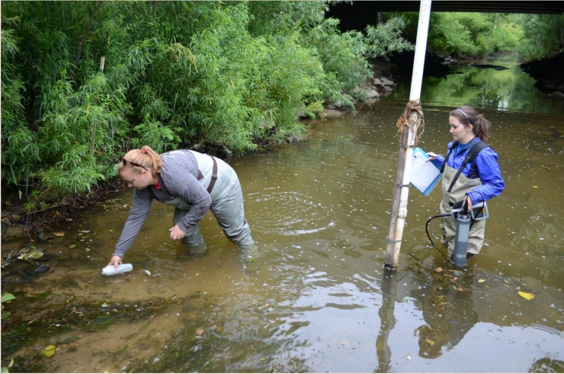
Figure 12: Nutrients and other key water quality parameters are measured upstream and downstream of the restoration areas during both dry and wet weather.
