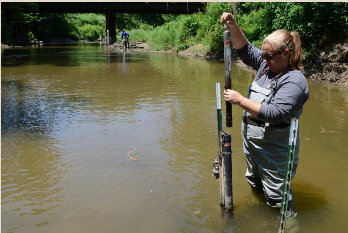
Figure 8: Regular maintenance of the turbidity sensors ensures they will collect high quality data that can be related to restoration activities, helping to document their effectiveness.
