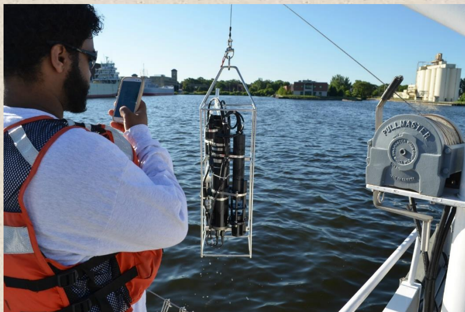
Figure 2: Sophisticated sensors are lowered through Muskegon Lake's water column to record water quality information that is used to characterize the lake's status.
